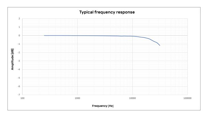
The frequency response is within ±3 dB up to 31.5 kHz
